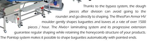
It is also possible after dividing to pass dough pieces into the rounder for a light rounding, before being shaped in the shaping machine, in particular for the production of special loaves, cut and short loaves and products requiring a little more body. The RheoPan line can produce at a rate of around 650Kg of dough per hour depending on the products. A new version with a larger head end should be available from the second half of 2020. It will be able to produce up to approximately 1000Kg /h.
