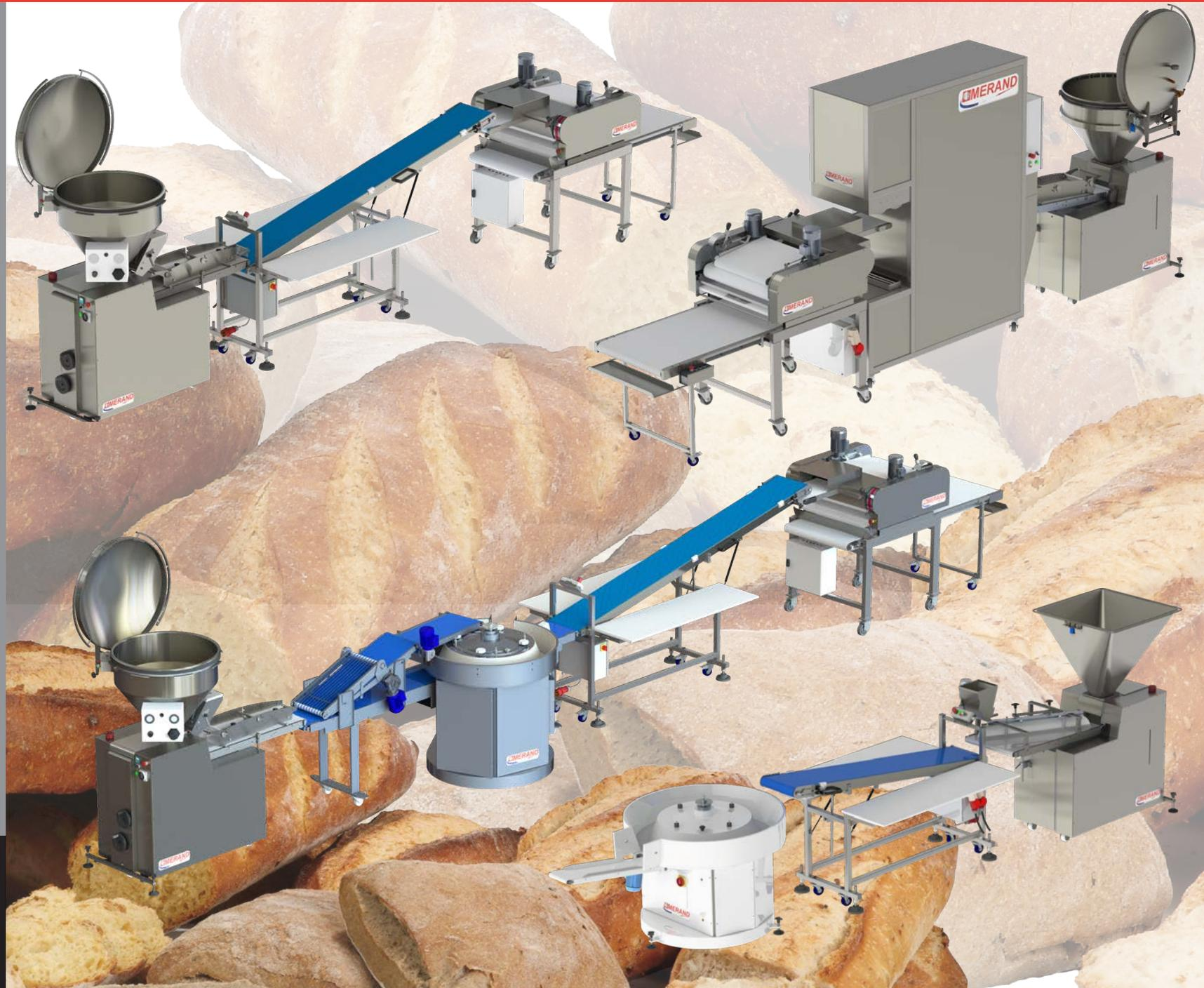
All EasyLine automatic production lines include a Softy piston automatic divider at the head end.
