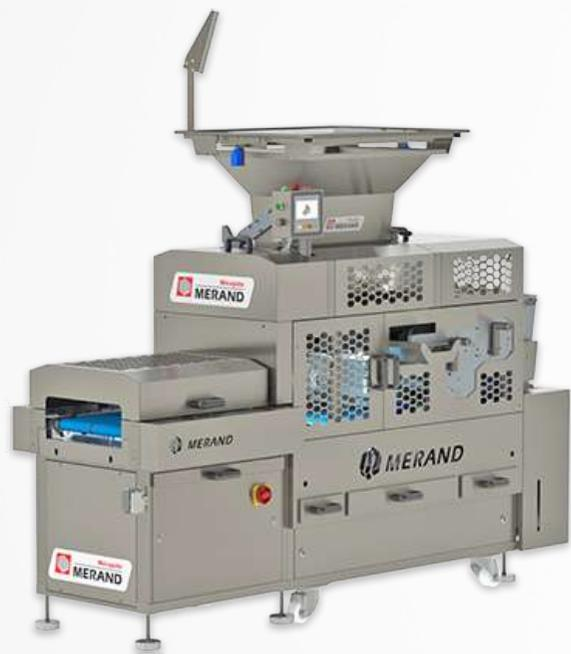
Its continuous double weighing system offers excellent regularity in weights, even when working with fermented dough. Each dough weight is controlled automatically on the second weighing belt. In case of a deviation from the target weight, the machine adjusts the settings automatically for cutting the next dough pieces.
