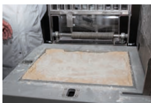
He closes the lid to spread the dough without degassing it thanks to the VarioPress®**
