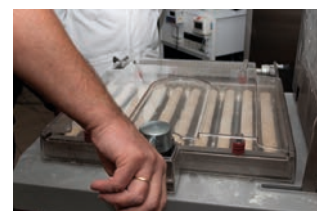
He chooses the right grid adapted to the dimensions of desired dough pieces and lifts the tray
