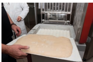
He reverses a dough block into the divider tank
