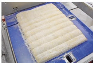
He reverses a dough block into the divider tank
